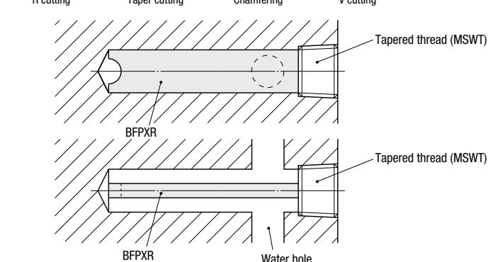
We recommend that the baffle board be lightly press-fitted into the cooling hole to prevent rotating.
