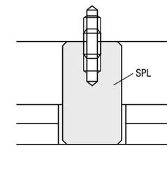
To fix the support pillar on a bottom clamping plate with a bolt.
