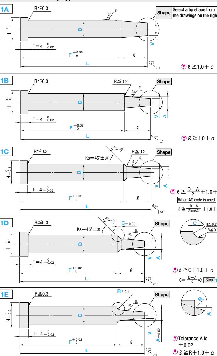
Shape (Tip shape: V is dimension before tip processing.)
