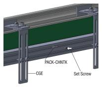
Position can be fixed with a nut alone by fastening the set screw included.
