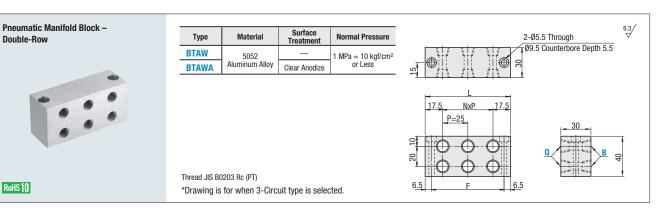
Features: Two-stage piping arrangement saves space in the horizontal direction.
