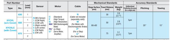
\*1. For motor options MA and PA, the driver is included in the set. For motor option U, the amplifier is included in the set. With motor options MA, PA and U, the selectable cable options are M, P and U, respectively and exclusively. Note that the cable option N is not selectable
