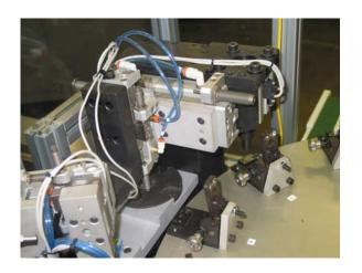
This section of a DTI machine, used to solder, assemble and test automotive ignition components, incorporates a majority of MISUMI parts, either standard or configured. Native CAD files can be downloaded in various formats (ProE, Inventor, IGES, et al.) directly into assemblies such as this one, thereby saving considerable design and development time.
