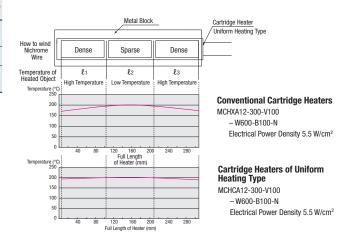
Heated Object: 303 Stainless Steel (30 x 30 x 300) Point of Temperature Measurement:  $\ell_1$ ,  $\ell_2$ ,  $\ell_3$  Center Part of Each Surface
