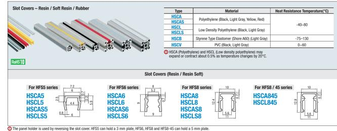
THISCL (Resin Soft) is softer than HSCA (Resin). Can be easily inserted after assembling the extrusions. (For details, see below. P.2903)
