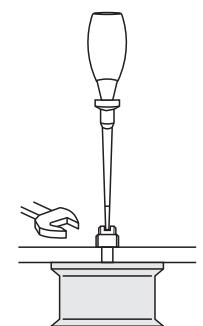
Tightening is possible by holding the threaded tip.
