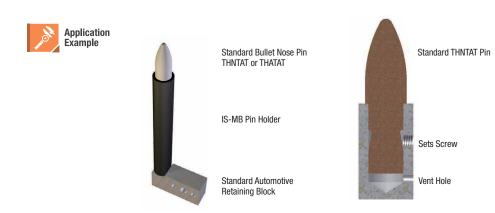
Misumi Automotive style Configurable pins (IS-NMF and IS-NML) are available with maximum head working length of 30 mm. In some situations, the location of the actual locating area requires a longer pin. The Pin Holder is designed to be used with THNTAT or THATAT style pins with set screw mount style configured as shown above.
