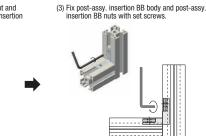
Features: Blind Brackets to connect Extrusions 45 / 30 square.
