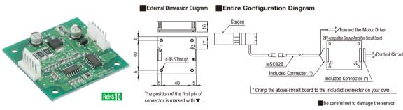
2. Establish the above connection in such way that it meets requirements for the control circuit you are to use.
