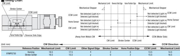
Homing Routine Above: When DS102/DS112 Series controller is used and when the Homing Routine Type 3 is executed. The coordinates shown are design values. There may be approx. ±0.5mm misalignment on the physical dimensions. For details about Homing, see P 1.735-97
