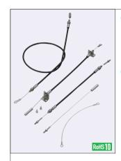
note: -25 to +80°C M Material: Wire Outer End (Threaded): 304 Stainless Steel Included Nut 4 pcs: (JIS Class 3): 304 Stainless Steel Outer Tube (Sheath): PVC (Black) Internal Liner: PF Inner Core Rod: Conner for Screw
