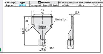
Part Number Orifice Weight (g) Applications: For removal of oil, water drops and chips, cooling/ drying and air curtain,
