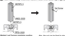
Welded Leaf Springs maintains position (even in vertical extrusions), leading to easy locating.
