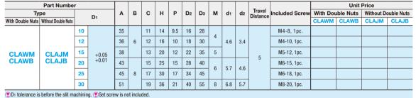
Recommended tolerances of fitting shafts for D1: g6, f8.
