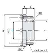
\* Thread diameter of screw hole for removal is the same as that of locking screw
