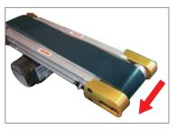
tensioning screw on the side the belt is deviated to.
