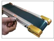
Slightly loosen 4 pulley holder mounting screws. (Take caution that the pulley may fall off if the screws are completely loosened.) Do the same for the other side.
