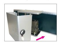
Next, adjust as shown previously with the Pulley Holder pensioning screw. As the belt Lateral movement decreases and the parallelism is confirmed, re-tighten the nut to complete.
