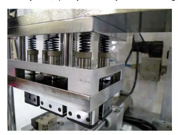
Basic press machine with a spring loaded head for assembling and pressing knobs onto a body.
